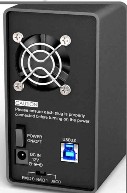
GR3660-B3 has three configuration modes built-in: RAID 1 (Safe Mode), RAID 0 (Speed Mode), and JBOD (Two Independent Volumes) for you to choose according to your needs.
